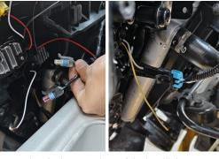
• Unplug the harness plugs of the headlights (fig.left) and DRL(fig.right).
