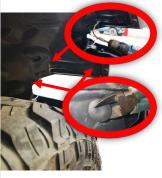
unscrew one screw and remove two plastic clips above the left/right front wheel from the inner lining.
