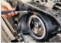
Adjust the tightness of the screws slightly to adjust the high and low beams.
